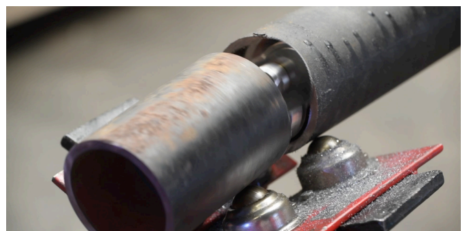
TCT® horizontal cutting result
